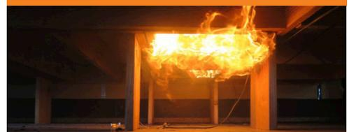
Narrow joist spacing was a condition that could result in fire growth in the under-deck area.
