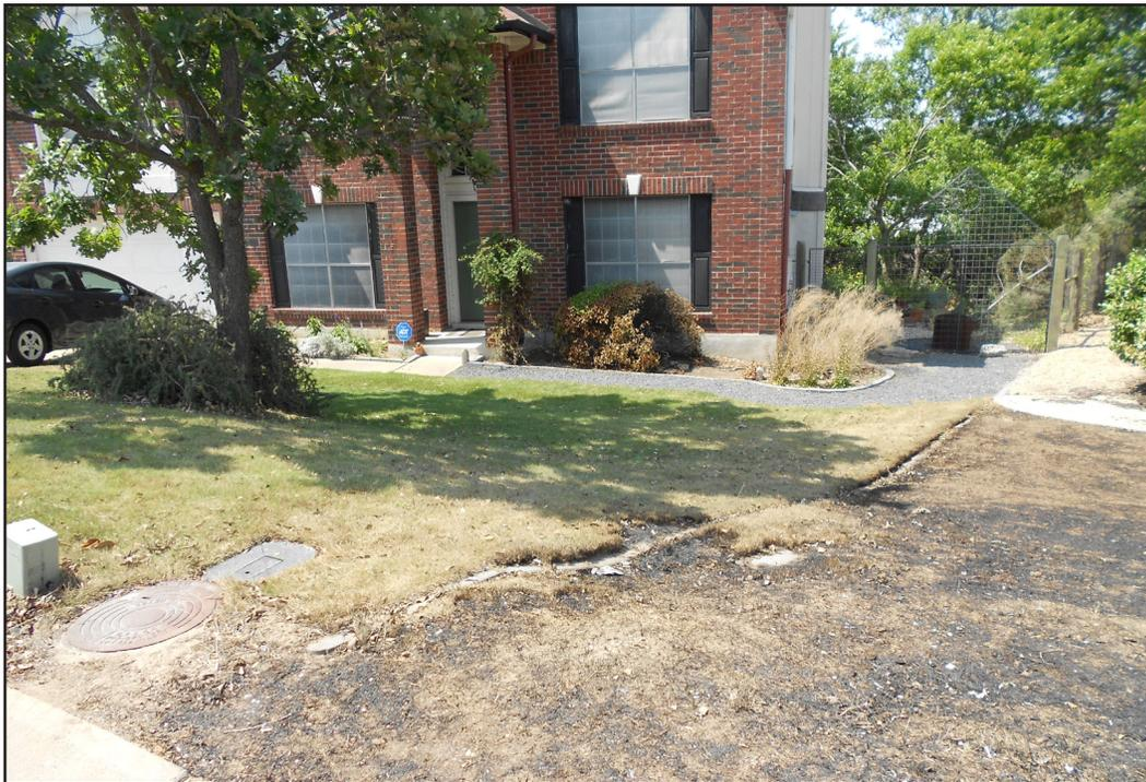
**The concrete driveway and gravel walkway created a critical space that firefighters needed to defend this home in the path of the Pinnacle Fire in Austin.**
