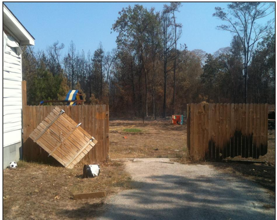
**This home on the Riley Road Fire didn't ignite because a portion of the attached fence was removed, preventing the fire from spreading to the house. Many other homes in the fire's path weren't as fortunate.**
