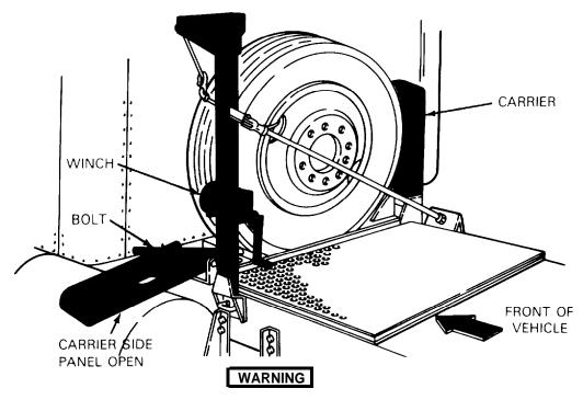
When paying out cable from the hoist, LEAVE FOUR FULL TURNS OF CABLE ON THE HOIST DRUM.
