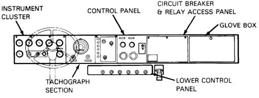
Figure 2-7. Instrument Panel.
