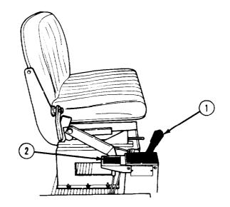
Figure 2-8. Transmission Range Selector Control and Sliding Fifth Wheel Control.
